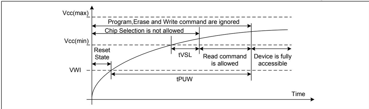
**Table3. Power-Up Timing and Write Inhibit Threshold**
