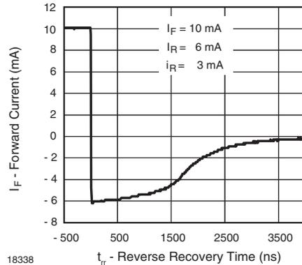
18338 Fig. 4 - Typical Charge Recovery Curve
