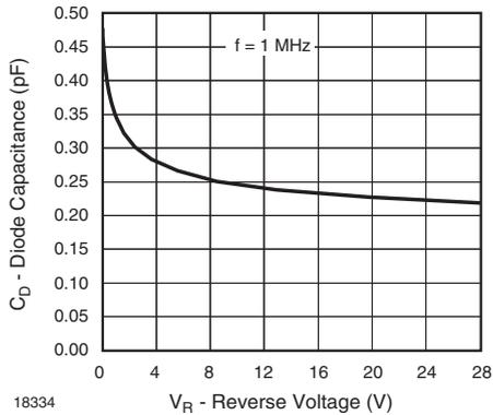
18334 Fig. 2 - Diode Capacitance vs. Reverse Voltage
