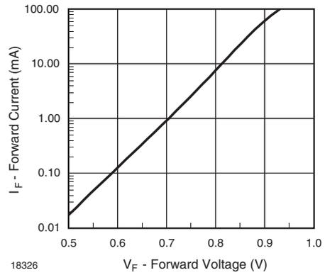
18326 Fig. 3 - Forward Current vs. Forward Voltage
