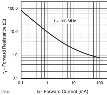
18342 Fig. 1 - Forward Resistance vs. Forward Current
