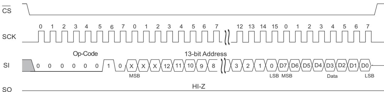
**Figure 14. Burst Mode Write Instruction Timing**
