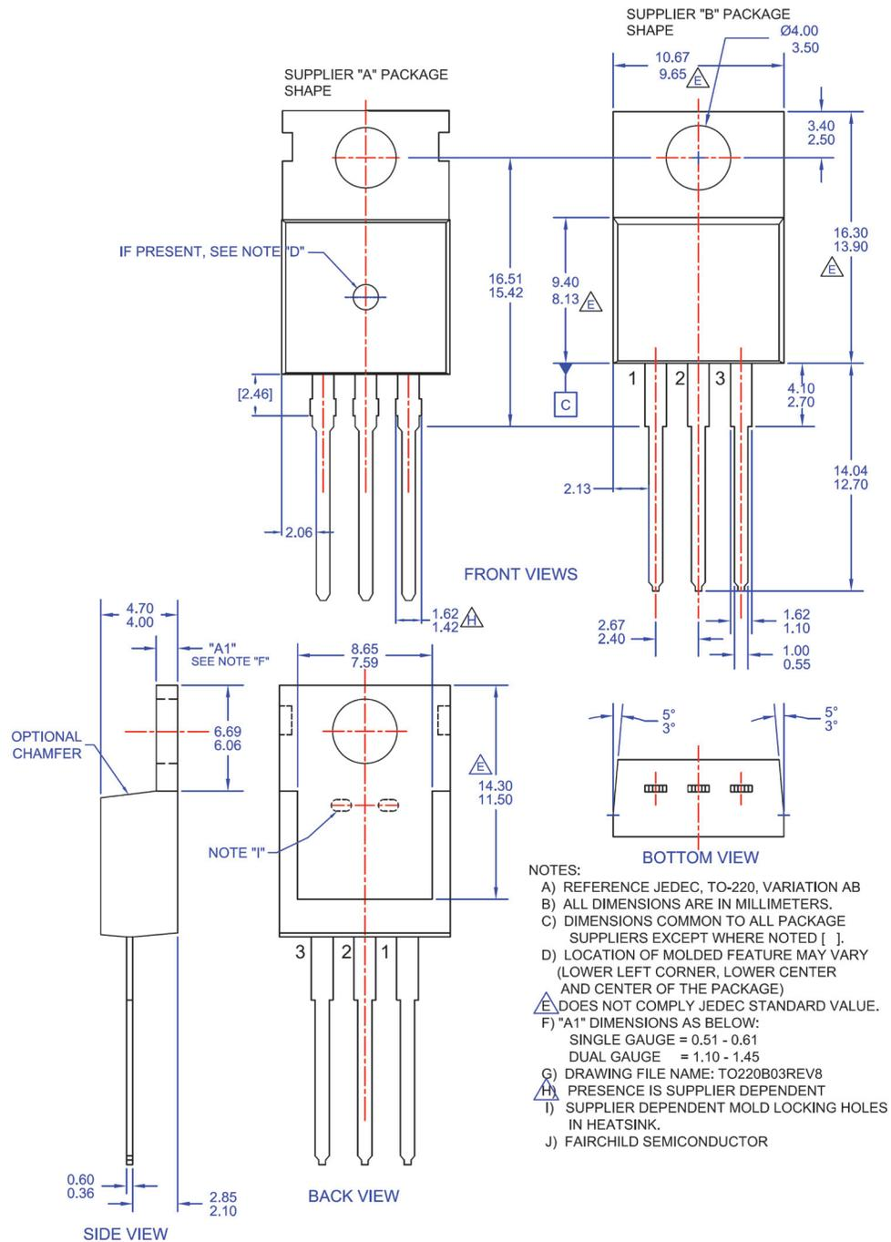
**Figure 16. TO220, Molded, 3-Lead, Non Jedec Variation AB**
