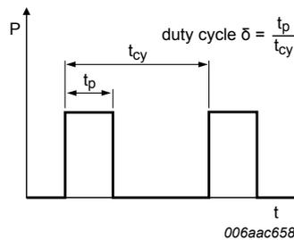
Fig. 17. Duty cycle definition
