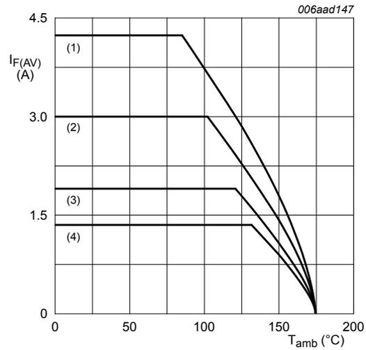
Ceramic PCB, Al<sub>2</sub>O<sub>3</sub>, standard footprint
