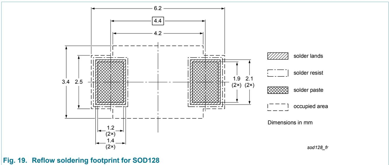
Fig. 19. Reflow soldering footprint for SOD128
