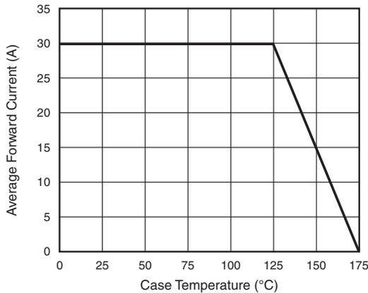
Fig. 1 - Forward Derating Curve Per Diode
