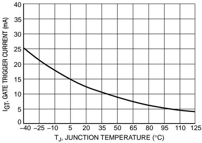
Figure 1. Typical Gate Trigger Current versus Junction Temperature
