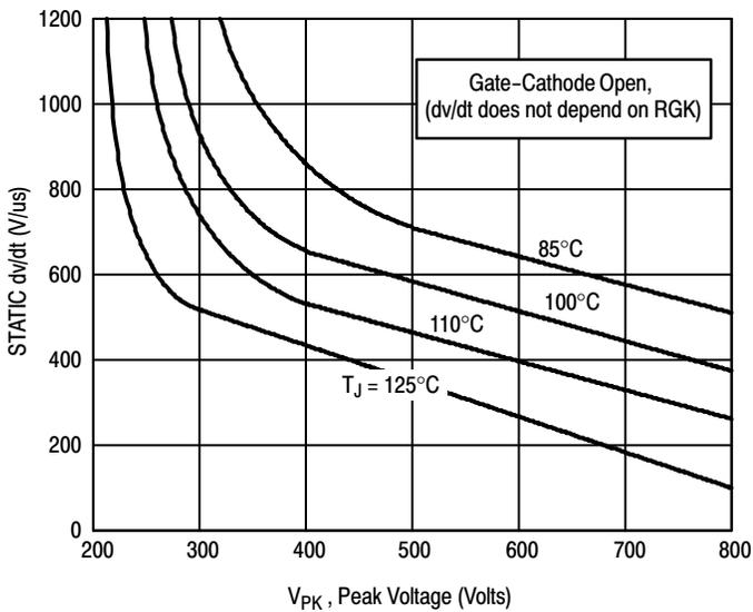
Figure 9. Typical Exponential Static dv/dt Versus Peak Voltage
