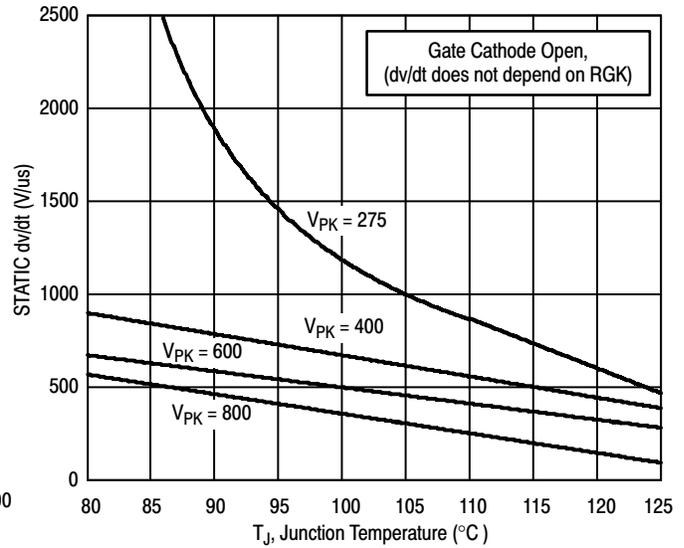
Figure 10. Typical Exponential Static dv/dt Versus Junction Temperature
