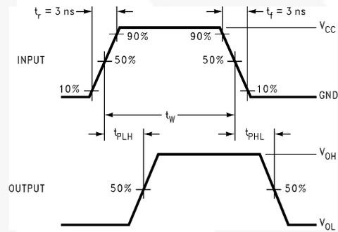
**Figure 5. AC Waveforms**
