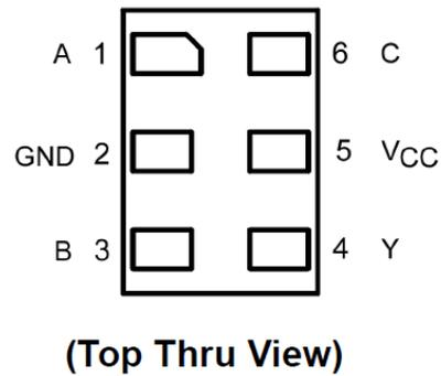
Figure 3. MicroPak (Top Through View)
