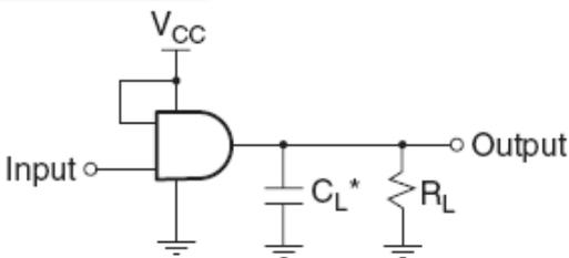
**Figure 4. AC Test Circuit**
