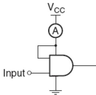
**Figure 6. I<sub>CCD</sub> Test Circuit**
