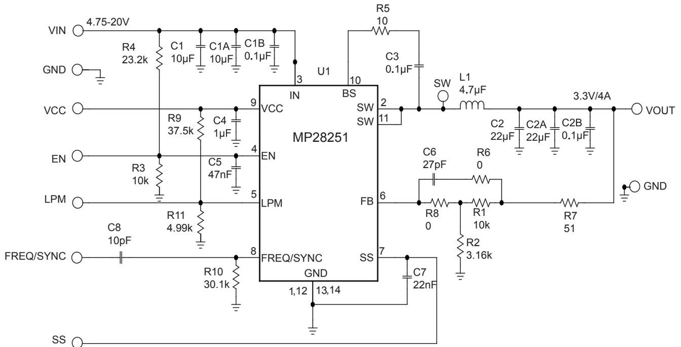
**Figure 6: 500kHz, 3.3V Output at 4A Step-Down Converter**
