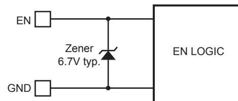
**Figure 2: Zener Diode between EN and GND**
