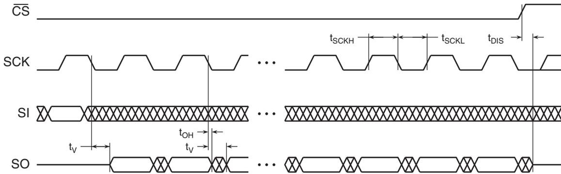
Figure 13-3. HOLD Timing – Serial Input
