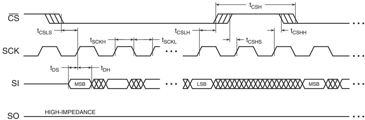
Figure 13-2. Serial Output Timing
