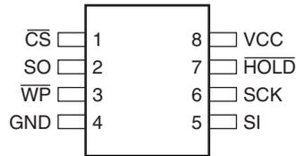
**Figure 2-2.** 16-SOIC Top View
