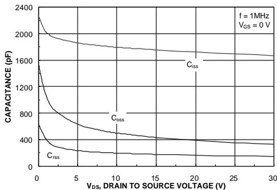
Figure 8. Capacitance Characteristics
