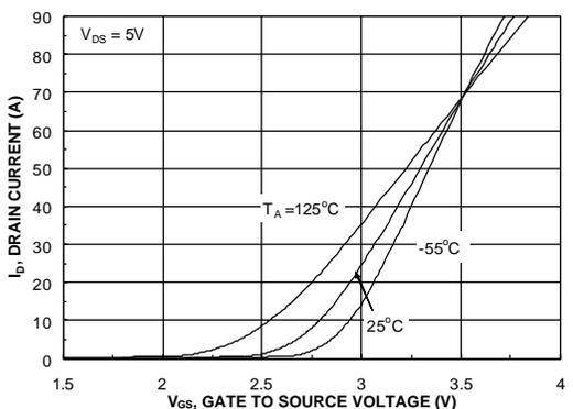
Figure 5. Transfer Characteristics
