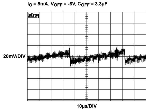
FIGURE 18.  $V_{OFF}$  RIPPLE
