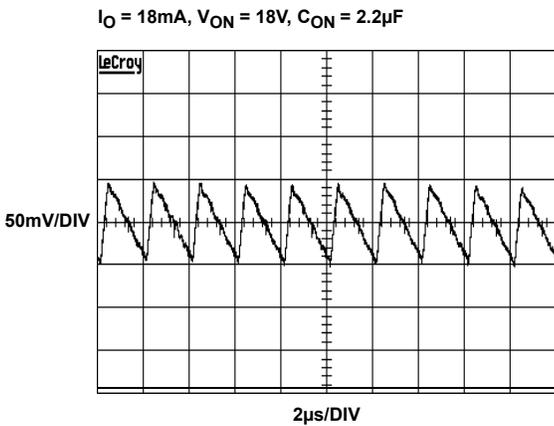
FIGURE 17.  $V_{ON}$  RIPPLE
