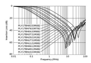
Common Mode Insertion Loss-Frequency Characteristics
