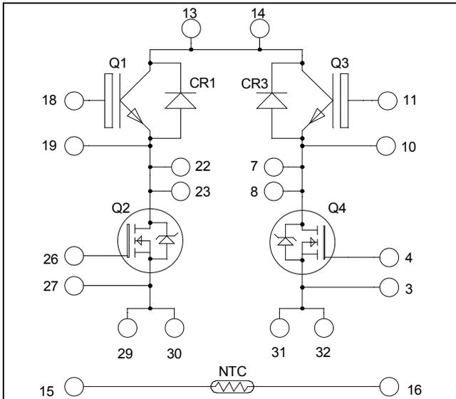
Top switches : Trench + Field Stop IGBT3
