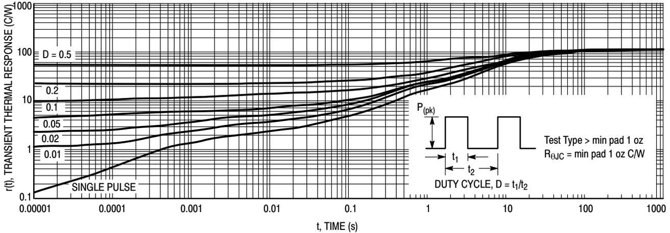
Figure 9. Thermal Response – MBRS540T3G, NRVBS540T3G on min pad
