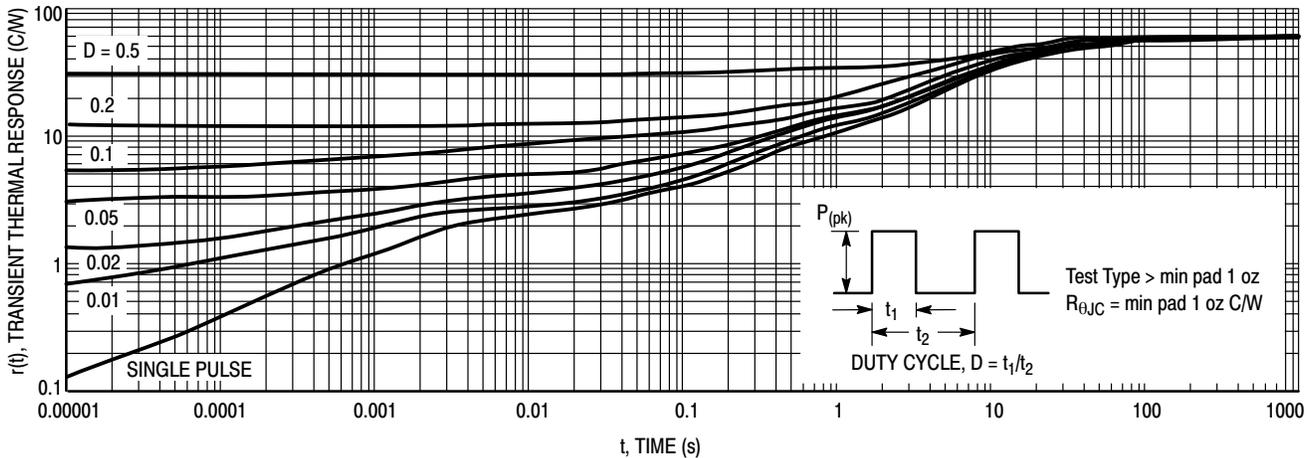
Figure 10. Thermal Response – MBRS540T3G, NRVBS540T3G on 1" pad
