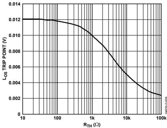
Figure 4. L<sub>05</sub> Trip Point vs. Threshold Adjust Resistor
