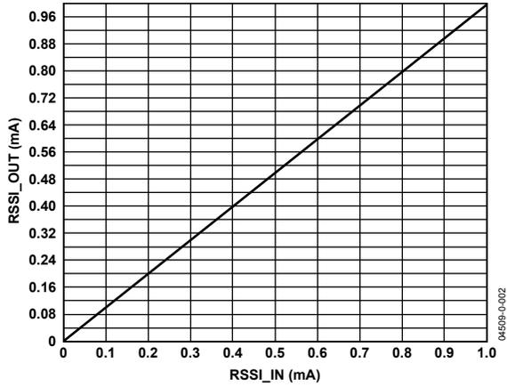
Figure 3. RSSI Output vs. Average PIN Photodiode Current
