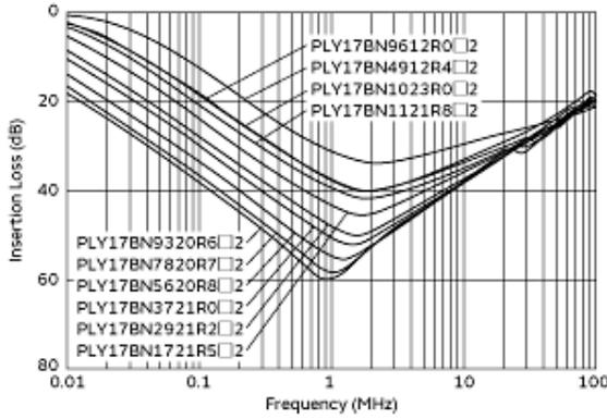
Common Mode Insertion Loss-Frequency Characteristics
