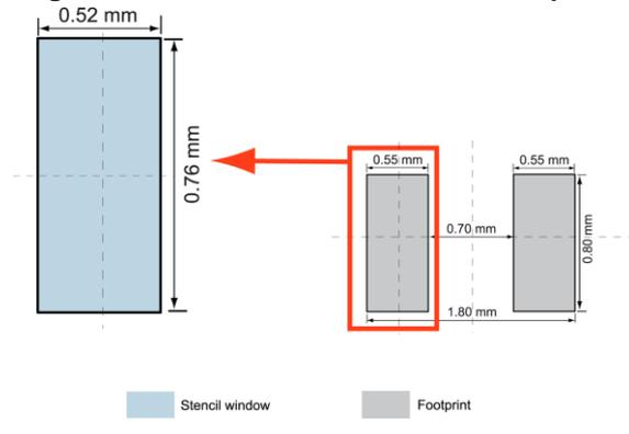
Figure 16: Alternative stencil window position
