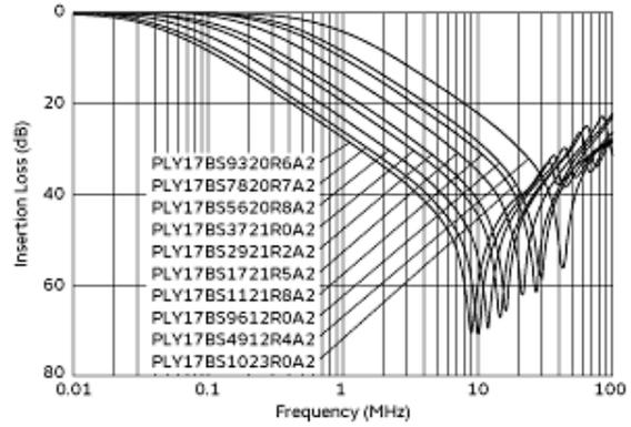
Differential Mode Insertion Loss-Frequency Characteristics
