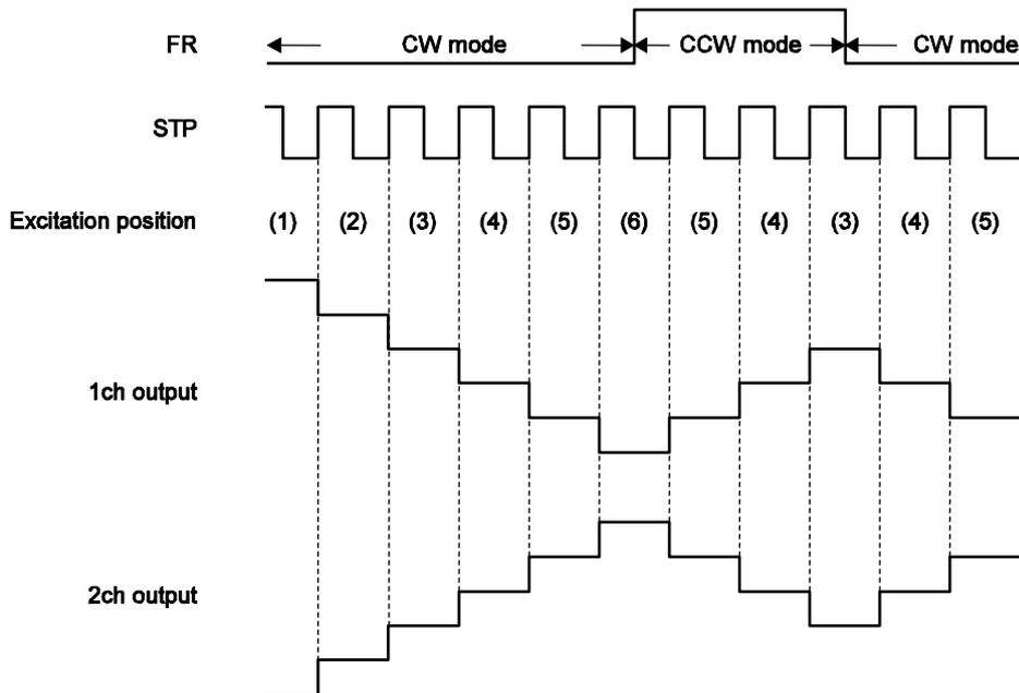
The internal D/A converter proceeds by one bit at the rising edge of the input STEP pulse. In addition, CW and CCW mode are switched by setting the FR pin. In CW mode, the channel 2 current phase is delayed by 90° relative to the channel 1 current. In CCW mode, the channel 2 current phase is advanced by 90° relative to the channel 1 current.
