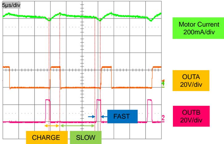
When the motor current reaches to the setting current, it is switched to Slow Decay mode.
