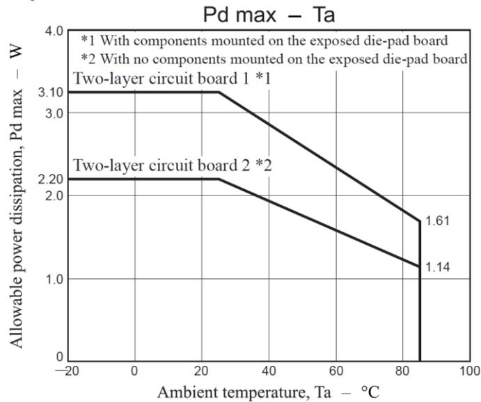
**Substrate Specifications** (Substrate recommended for operation of LV8746V)
