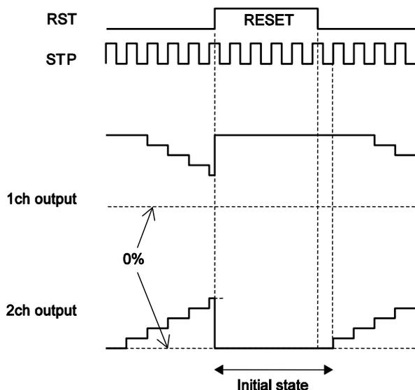
When the RST pin is set to High, the excitation position of the output is forcibly set to the initial state. When RST is then set to Low, the excitation position is advanced by the next STP input.
