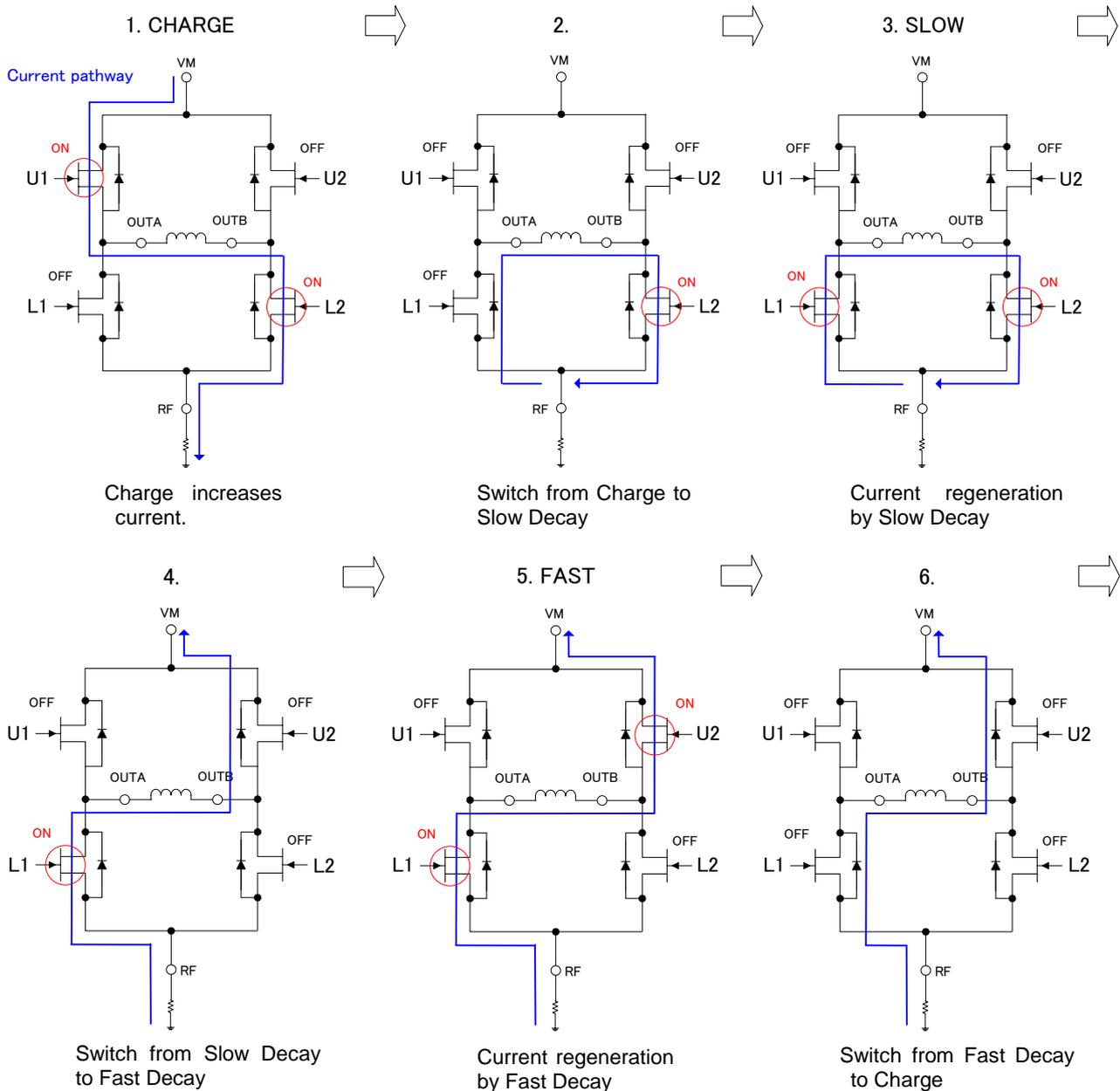
This IC controls constant current by performing chopping to output transistor.
