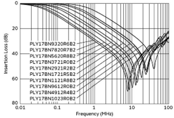
Differential Mode Insertion Loss-Frequency Characteristics
