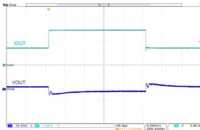
Figure 16. Load Transient, 3.6  $V_{IN}$ , 1.15625  $V_{OUT}$ , 1.5-3 A, 120 ns Edge
