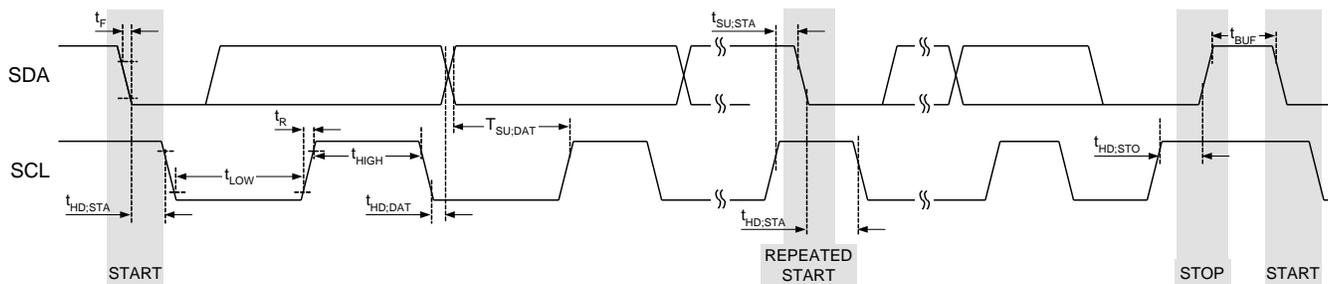
**Figure 4. I<sup>2</sup>C Interface Timing for Fast Plus, Fast, and Slow Modes**
