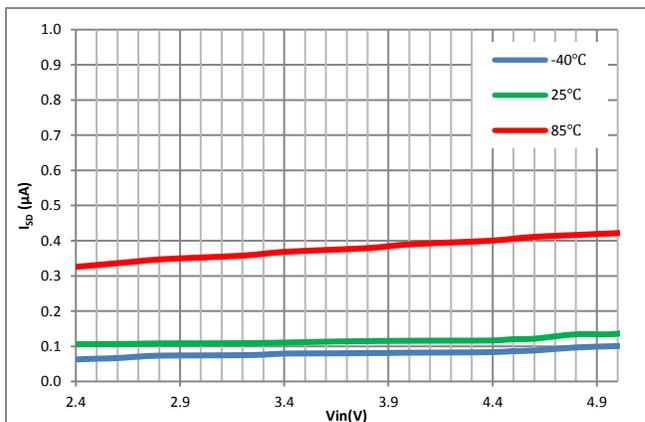
Figure 13. Shutdown Current vs. Input Voltage and Temperature
