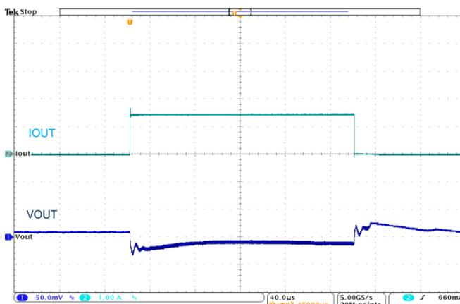
Figure 15. Load Transient, 3.6  $V_{IN}$ , 1.15625  $V_{OUT}$ , 0.01-1.5 A, 120 ns Edge
