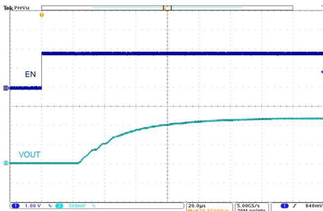
Figure 17. Startup, 5  $\Omega$  Load,  $V_{OUT}=1.15625\text{ V}$ ,  $V_{IN}=3.6\text{ V}$
