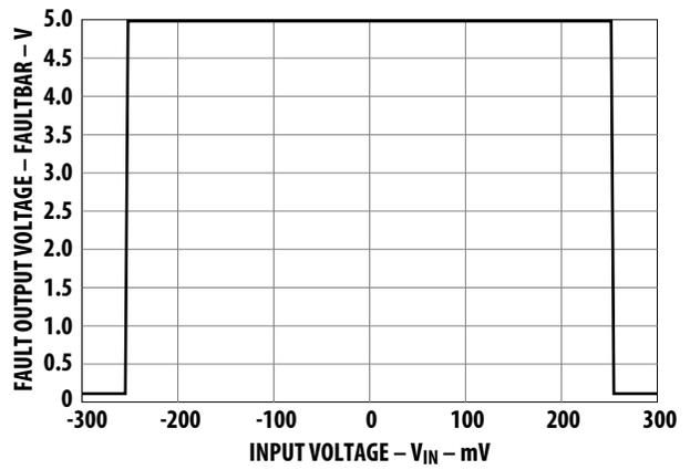
Figure 10.  $\overline{\text{FAULT}}$  output voltage vs.  $V_{IN}$ .
