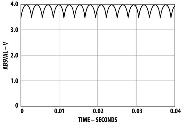
Figure 22. ABSVAL with 3 phases, wired-ORed together.
