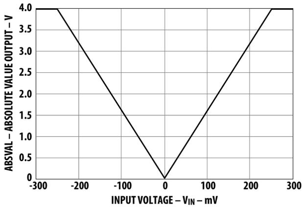
Figure 11. ABSVAL output voltage vs.  $V_{IN}$ .
