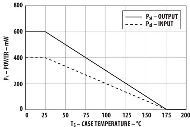
Figure 2. Dependence of safety-limiting values on temperature.
