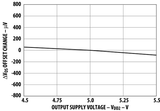
Figure 5. Input offset voltage change vs.  $V_{DD2}$ .
