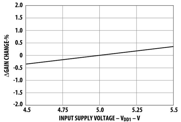
Figure 8. Gain change vs.  $V_{DD1}$ .
