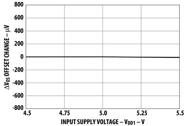
Figure 4. Input offset voltage change vs.  $V_{DD1}$ .
