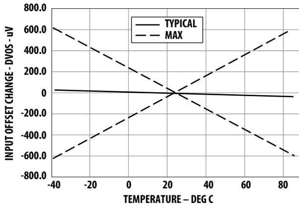
Figure 3. Input offset voltage change vs. temperature.
