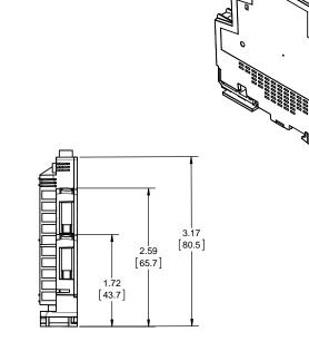
Tolerances: ± 0.02 in / 0.5 mm. All dimensions are in: inches [millimeters]
