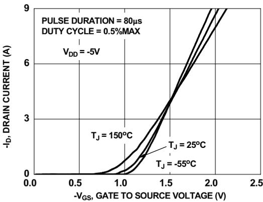
**Figure 5. Transfer Characteristics**
