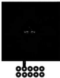
a.  $170^\circ\text{C}/\text{W}$  when mounted on a  $1\text{in}^2$  pad of 2 oz copper.
