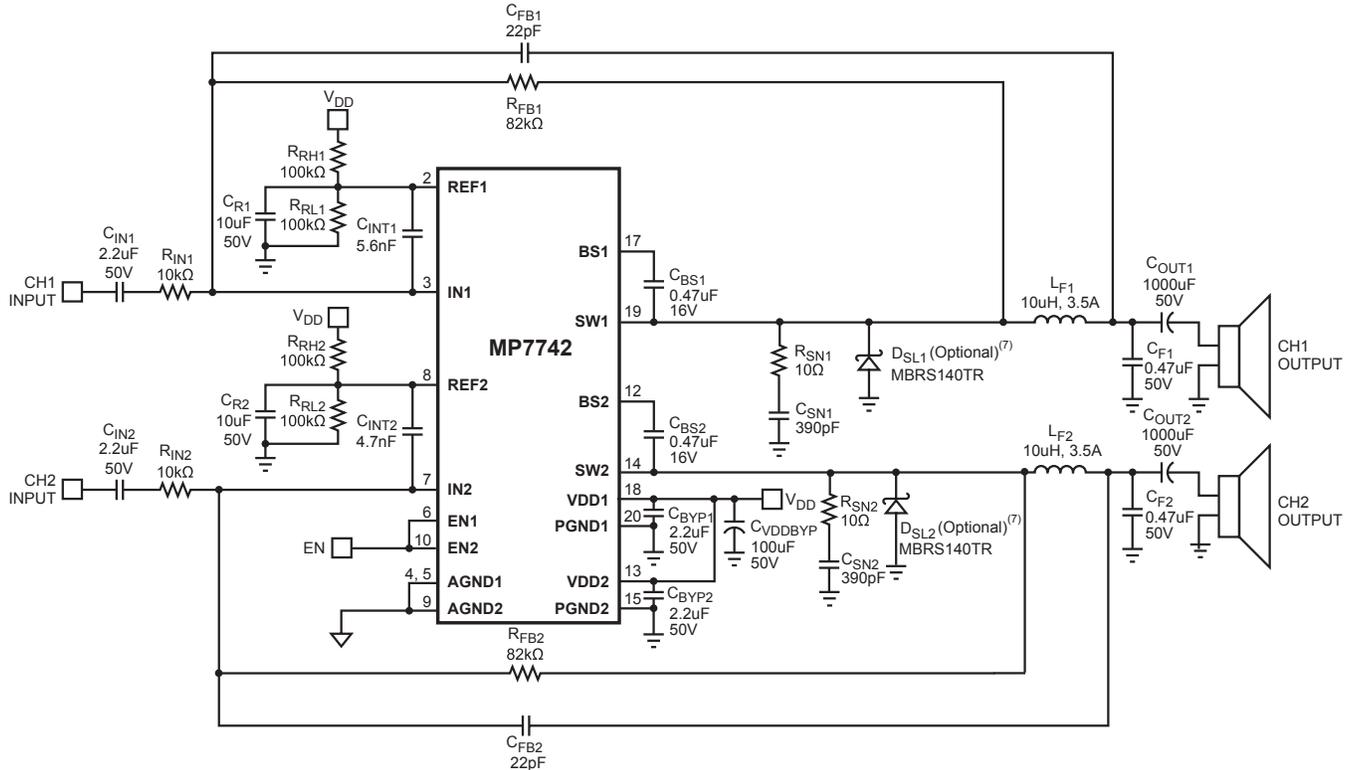
**Figure 1—2 x 15W Stereo Typical Application Circuit**
