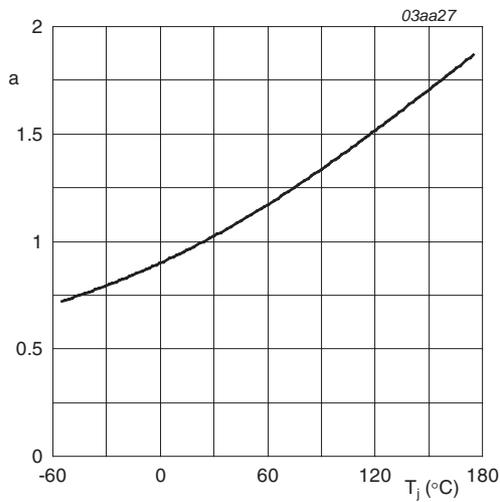
$$a = \frac{R_{DSon}}{R_{DSon(25^\circ\text{C})}}$$
