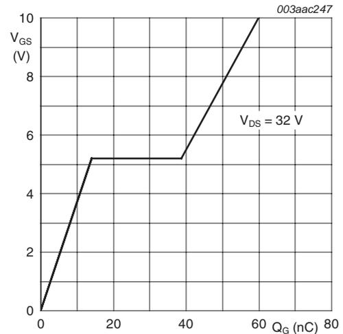
$T_j = 25\text{ }^\circ\text{C}; I_D = 25A$
