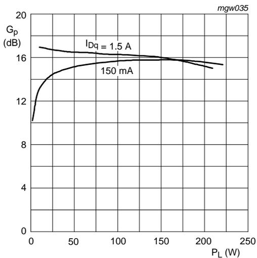
$V_{DS} = 36 \text{ V}$ ;  $f = 1060 \text{ MHz}$ ;  $t_p = 50 \text{ }\mu\text{s}$ ;  $\delta = 2 \text{ \%}$
