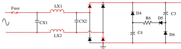
Figure 7: Stage A of Valley Fill Circuit
