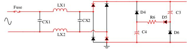
Figure 8: Stage B of Valley Fill Circuit
