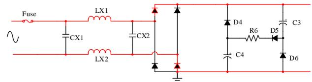
Figure 9: Stage C of Valley Fill Circuit
