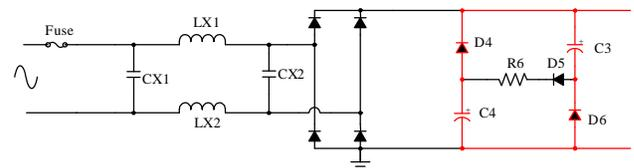
**Figure 10: Stage D of Valley Fill Circuit**
