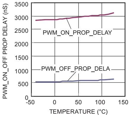
**DIM\_PWM\_INPUT vs. Temp**
