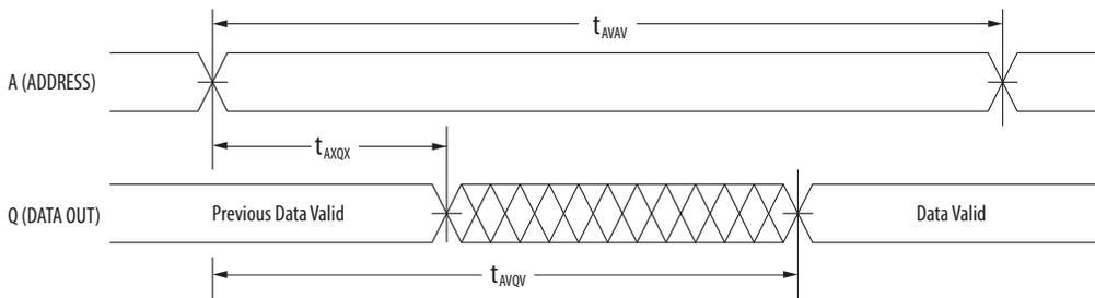
NOTE: Device is continuously selected ( $\bar{E} \leq V_{IL}, \bar{G} \leq V_{IL}$ )
