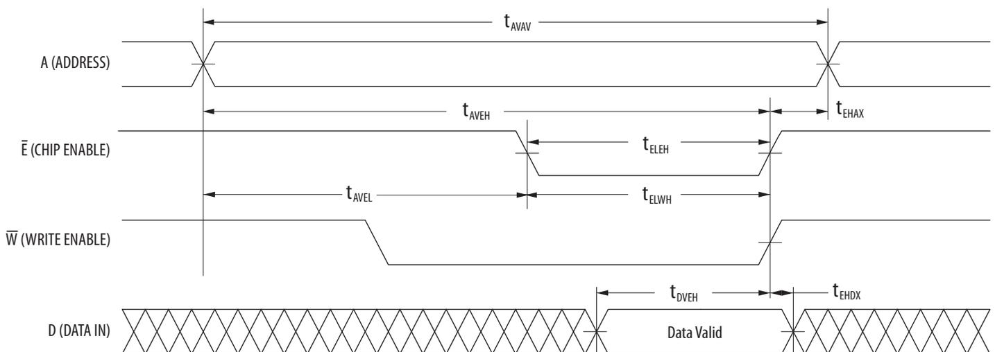
**Table 3.6 Write Cycle Timing 3 (Shortened  $t_{WHAX}$ ,  $\bar{W}$  and  $\bar{E}$  Controlled)<sup>1</sup>**
