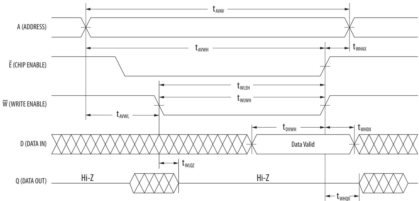
Table 3.5 Write Cycle Timing 2 ( $\bar{E}$  Controlled)<sup>1</sup>
