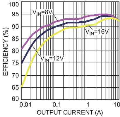
Figure 44 — Efficiency Curve
