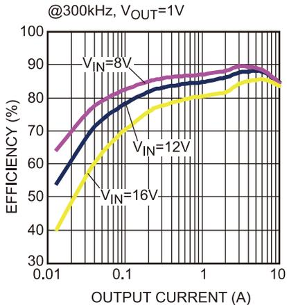
**Figure 18 — Efficiency Curve**
