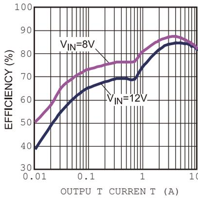
Figure 20 — Efficiency Curve
