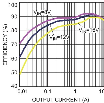
Figure 38 — Efficiency Curve
