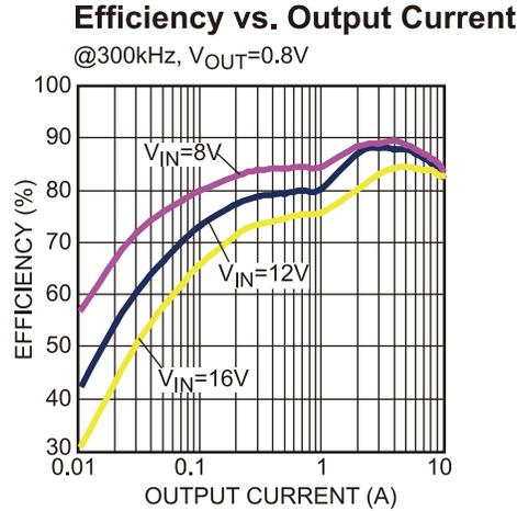
**Figure 22 — Efficiency Curve**
