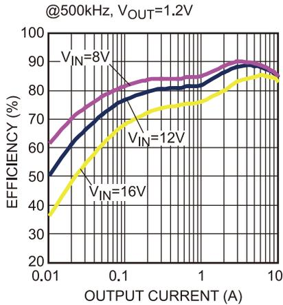
**Figure 28 — Efficiency Curve**
