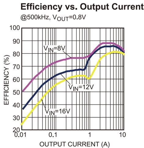
**Figure 24 — Efficiency Curve**
