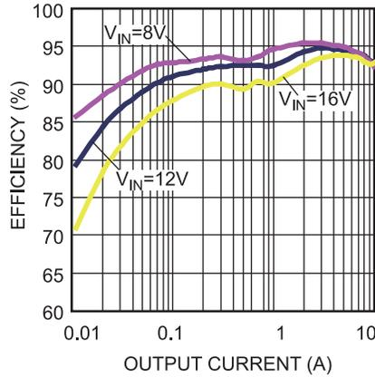
**Figure 52 — Efficiency Curve**
