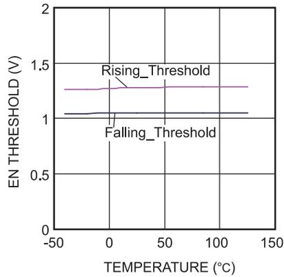
**V<sub>CC</sub> UVLO Threshold vs. Temperature**
