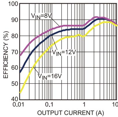
Figure 32 — Efficiency Curve
