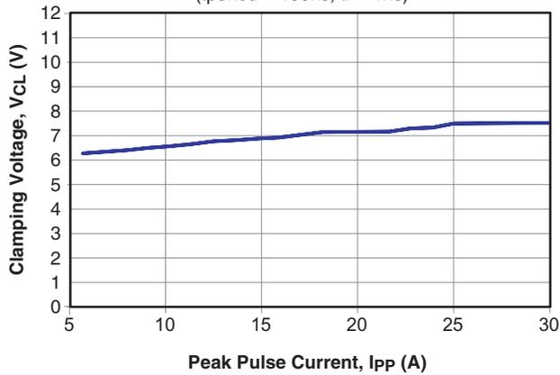
**Clamping Voltage vs. Current**
