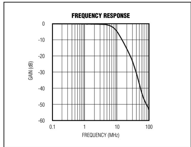
Figure 4. Frequency Response for 2nd-Order Lowpass Filter
