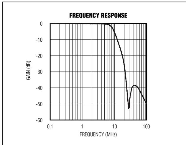
Figure 6. Frequency Response for 3rd-Order Lowpass Filter
