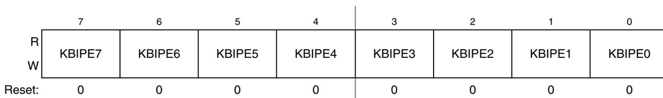
Figure 7-4. KBI Interrupt Pin Select Register (KBIXPE)
