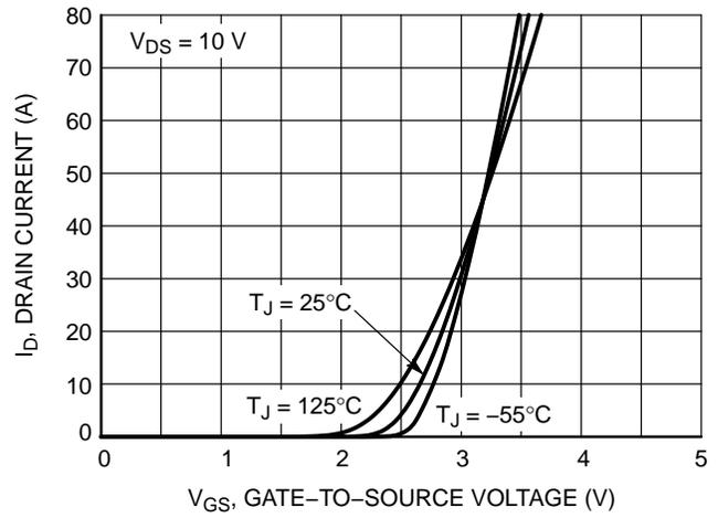
Figure 2. Transfer Characteristics
