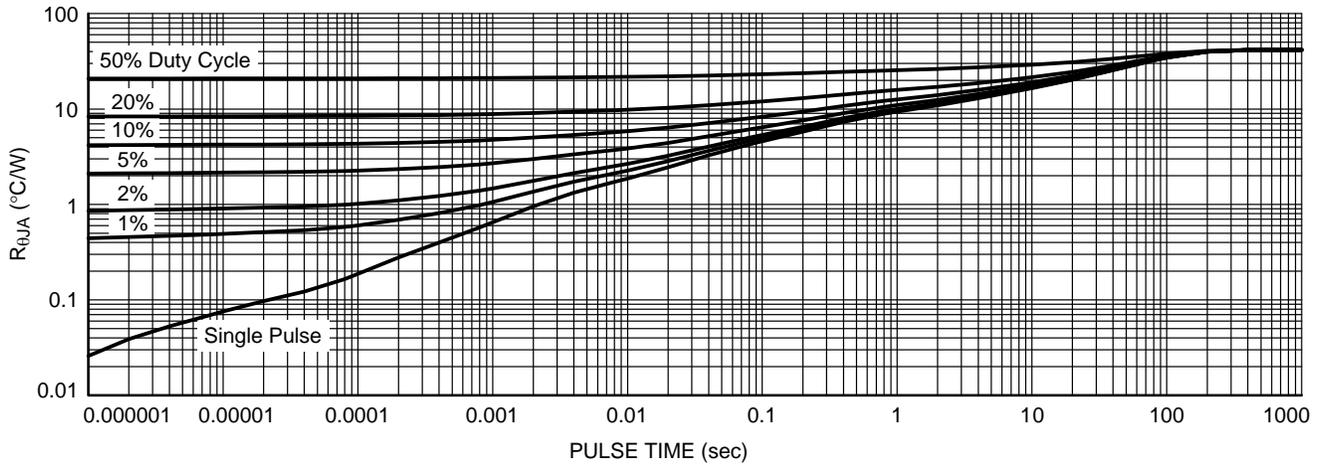
Figure 13. Thermal Characteristics
