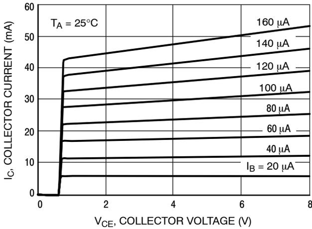
Figure 1.  $I_C - V_{CE}$
