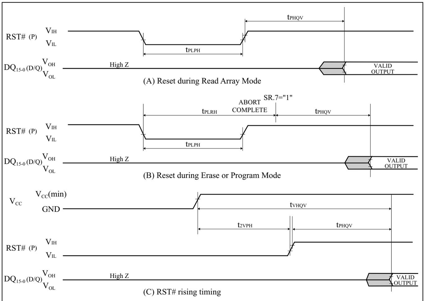
Figure 8. AC Waveform for Reset Operations
