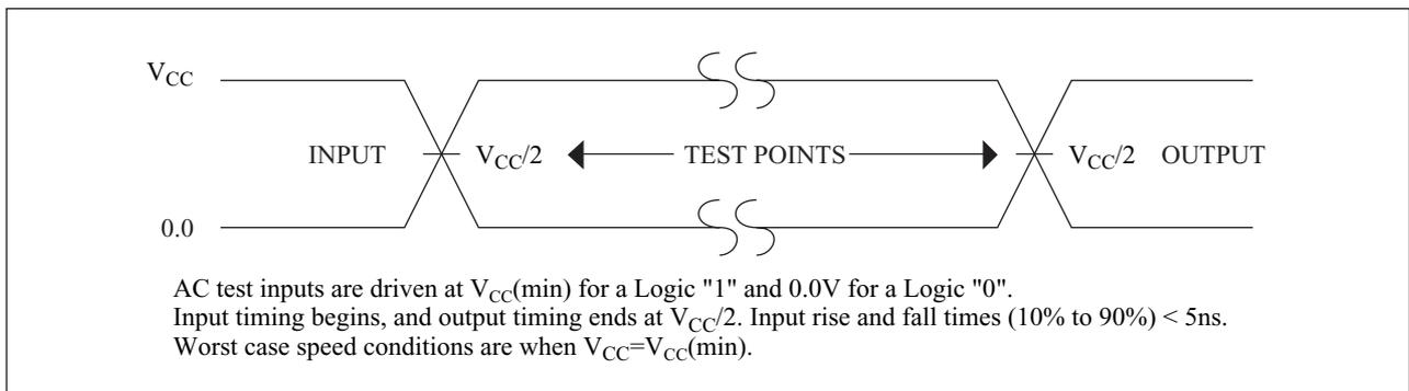
Figure 4. Transient Input/Output Reference Waveform for  $V_{CC}=2.7\text{V}-3.6\text{V}$
