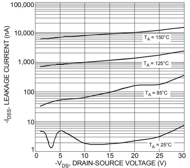
Figure 10 Typical Leakage Current vs. Drain-Source Voltage
