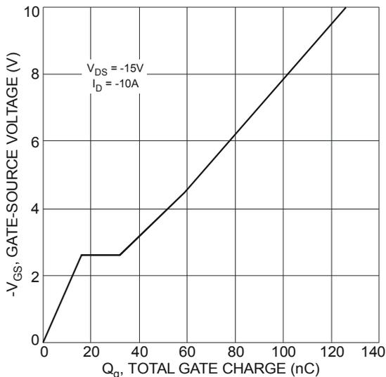
Figure 11 Gate-Source Voltage vs. Total Gate Charge
