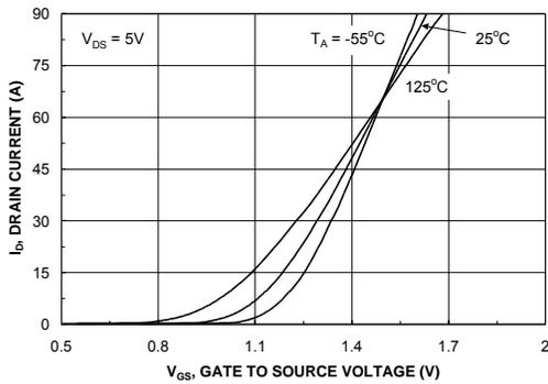
Figure 5. Transfer Characteristics.
