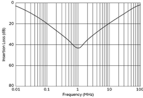
Common Mode Insertion Loss (Typ.)
