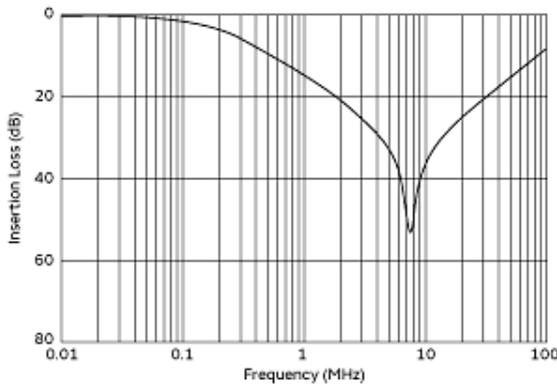
Differential Mode Insertion Loss (Typ.)
