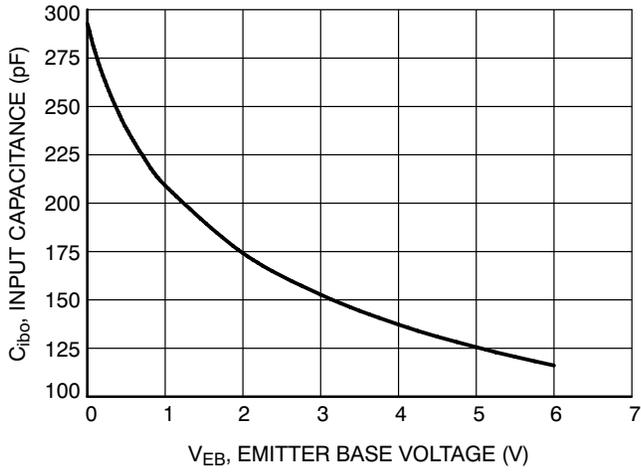
**Figure 21. Input Capacitance**
