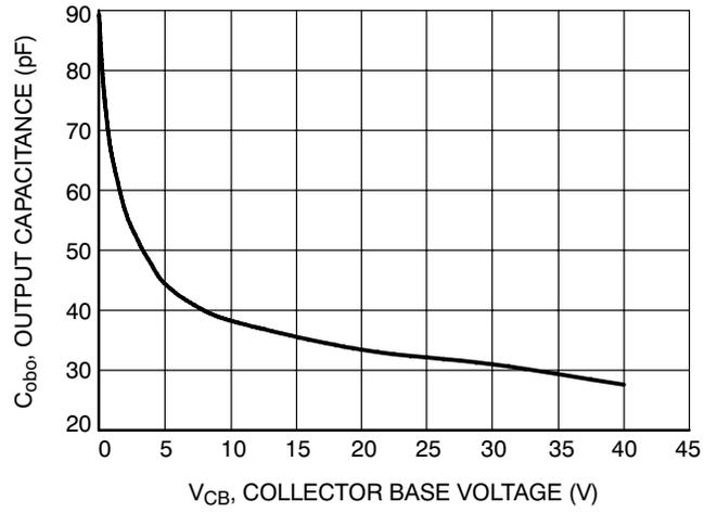
**Figure 22. Output Capacitance**
