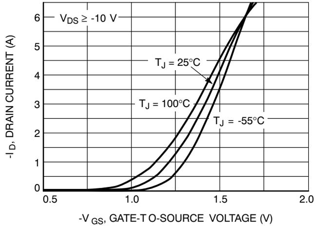
Figure 4. Transfer Characteristics
