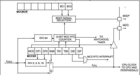
Figure 41. Main clock controller (MCC/RTC) block diagram
