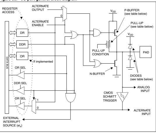
Figure 35. I/O port general block diagram
