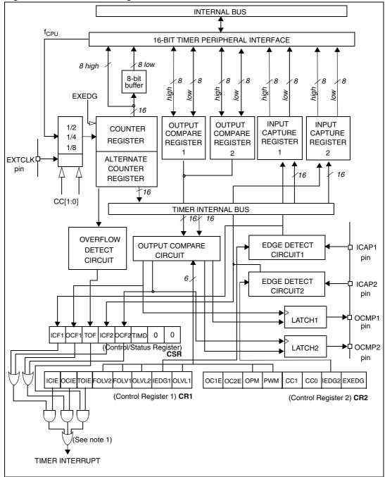
Figure 42. Timer block diagram
