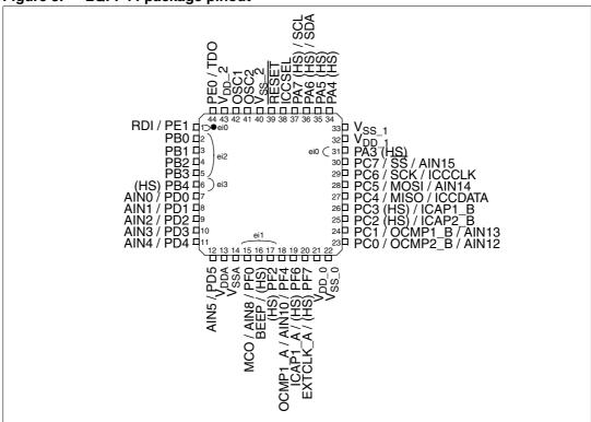
Figure 3. LQFP44 package pinout
