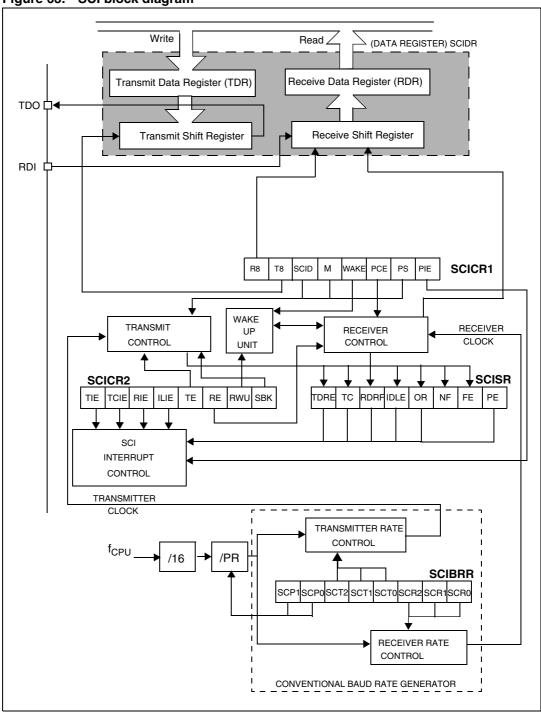
Figure 63. SCI block diagram
