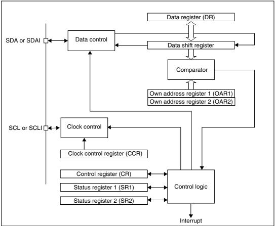
Figure 68. I<sup>2</sup>C interface block diagram
