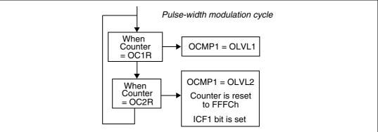
If OLVL1=1 and OLVL2=0 the length of the positive pulse is the difference between the OC2R and OC1R registers.
