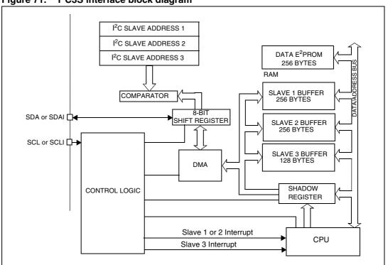
Figure 71. I<sup>2</sup>C3S interface block diagram
