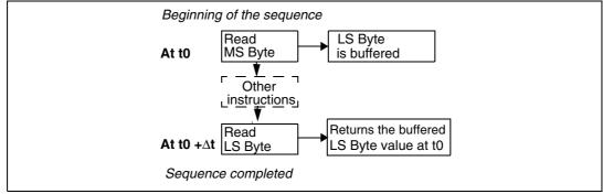
The user must read the MS Byte first, then the LS Byte value is buffered automatically.
