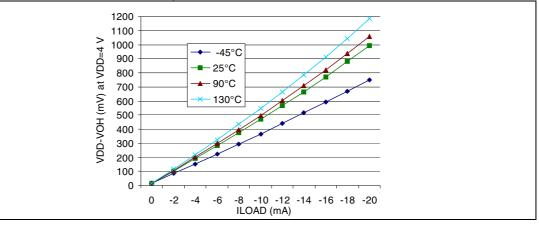
Figure 113. Typical  $V_{DD} - V_{OH}$  at  $V_{DD} = 5 V$  (std)
