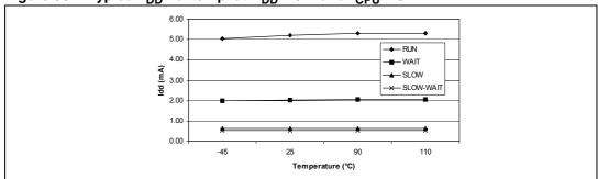
Figure 95. Typical I<sub>DD</sub> vs. temp. at  $V_{DD}$  = 5 V and  $f_{CPU}$  = 8 MHz
