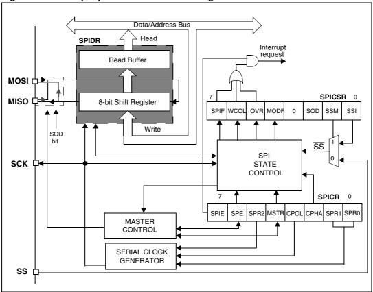
Figure 56. Serial peripheral interface block diagram
