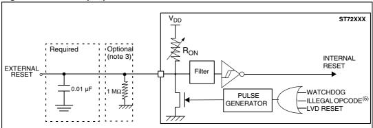
Figure 115. RESET pin protection when LVD is enabled  $^{(1)(2)(3)(4)}$
