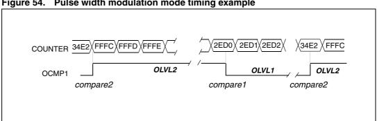
Figure 54. Pulse width modulation mode timing example
