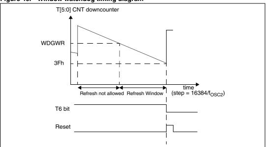
Figure 40. Window watchdog timing diagram
