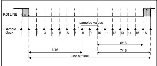
Figure 66. Bit sampling in reception mode
