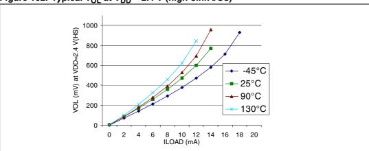
Figure 102. Typical V<sub>OL</sub> at V<sub>DD</sub> = 2.4 V (high-sink I/Os)
