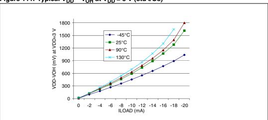
Figure 111. Typical  $V_{DD} - V_{OH}$  at  $V_{DD} = 3 V$  (std I/Os)
