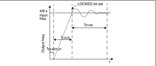
When the PLL is started, after reset or wakeup from Halt mode or AWUFH mode, it outputs the clock after a delay of t<sub>STARTUP</sub>
