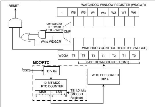
Figure 37. Watchdog block diagram
