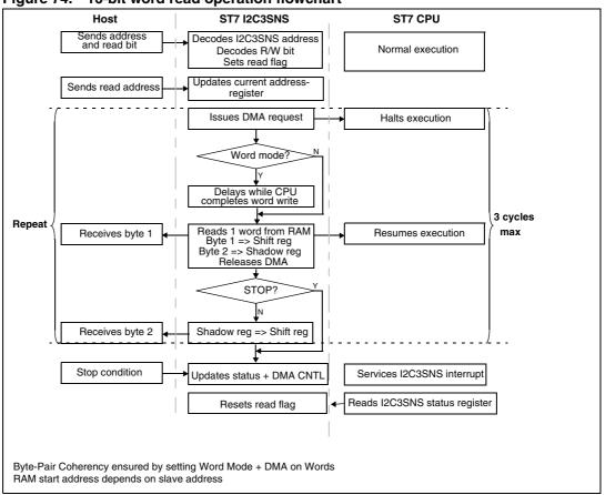
Figure 74. 16-bit word read operation flowchart
