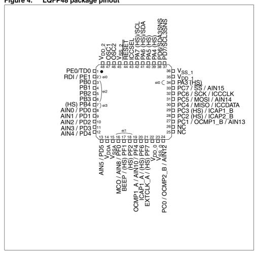
Figure 4. LQFP48 package pinout
