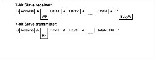
Legend: S = Start, P = Stop, A = Acknowledge, NA = Non-acknowledge, WF = WF event, WFx bit is set (with interrupt if ITWEx=1, after Stop or Restart conditions), cleared by reading the I2C3SSR register while no communication is ongoing.
