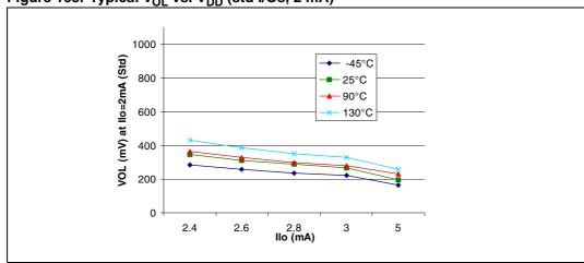
Figure 105. Typical V<sub>OL</sub> vs. V<sub>DD</sub> (std I/Os, 2 mA)
