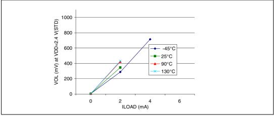
Figure 101. Typical  $V_{OL}$  at  $V_{DD}$  = 5 V (std I/Os)
