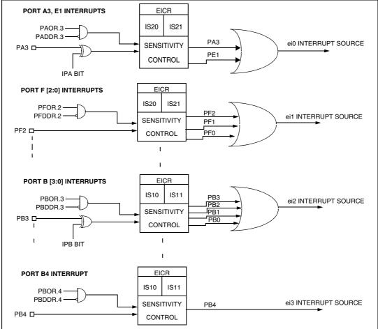
Figure 24. External interrupt control bits
