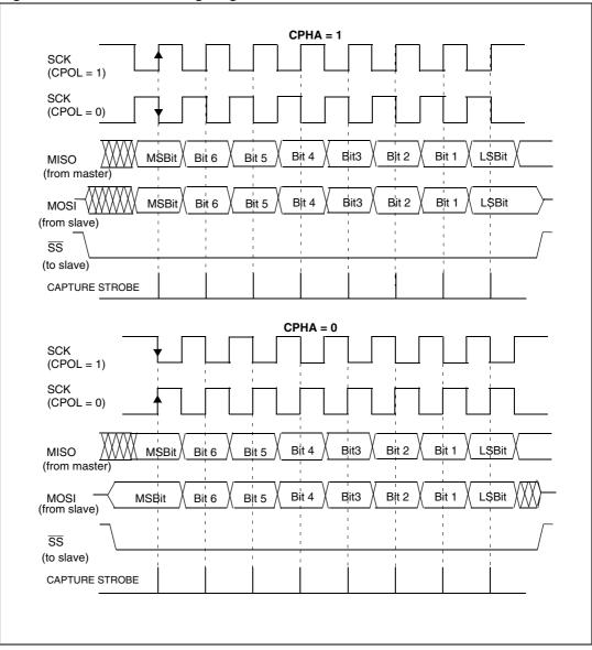
Figure 60. Data clock timing diagram
