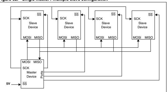
Figure 62. Single master / multiple slave configuration
